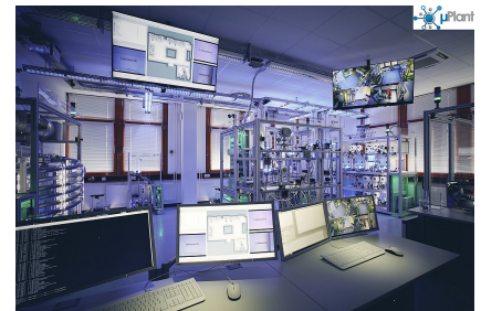
Figure 1: Small-scale factory \mu Plant
