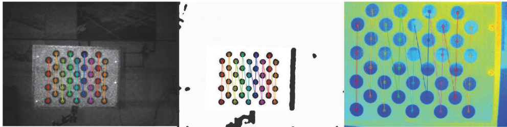
Figure 1: Calibration target in the near infrared range (l.), depth image (m.) and infrared (r.).
